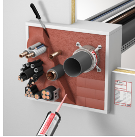
Fig. 2: Installation in flexible wall
