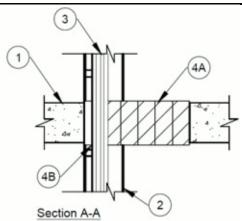
1. **Floor or Wall Assembly** — Min 4-1/2 in. (114 mm) thick reinforced lightweight or normal weight (100-150 pcf or 1600-2400 kg/m<sup>3</sup>) concrete. Wall may also be constructed of any UL Classified **Concrete Blocks\*.** Max area of opening is 384 in.<sup>2</sup> (2477 cm<sup>2</sup>) with a max dimension of 32 in. (813 mm).
