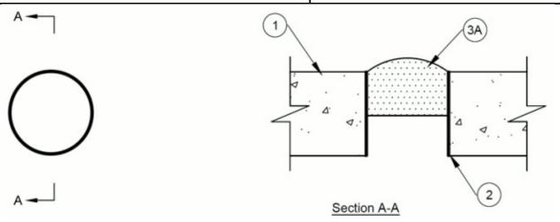
1. **Floor or Wall Assembly** — Min 4-1/2 in. (114 mm) thick reinforced lightweight or normal weight (100-150 pcf or 1600-2400 kg/m<sup>3</sup>) concrete. Wall may also be constructed of any UL Classified **Concrete Blocks\*.** Max diameter of opening is nom, 5 in. (127 mm).
