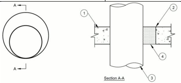
1. **Floor or Wall Assembly** — Min 4-1/2 in. (114 mm) thick reinforced lightweight or normal weight (100 - 150 pcf or 1600-2400 kg/m<sup>3</sup>) concrete. Wall may also be constructed of any UL Classified **Concrete Blocks\*.** Max diam of opening is 12 in. (305 mm).
