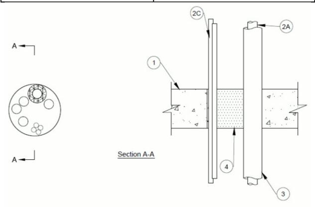
$1600-2400 \text{ kg/m}^3$ ) concrete. Wall may also be constructed of any UL Classified **Concrete Blocks\*.** Max diam of opening is 6 in. (0.15 m).
