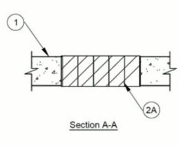
1. **Floor or Wall Assembly** — Min 4-1/2 in. (114 mm) thick reinforced lightweight or normal weight (100-150 pcf or 1600-2400 kg/m³) concrete. Wall may also be constructed of any UL Classified **Concrete Blocks\*.** Max area of opening is 384 in.² (2477 cm²) with a max dimension of 32 in. (813 mm).
