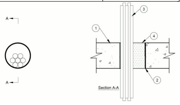
1. Floor or Wall Assembly — Min 4-1/2 in. (114 mm) thick reinforced lightweight or normal weight (100-150 pcf or  $1600 - 2400 \text{ kg/m}^3$ ) concrete. Wall may also be constructed of any UL Classified **Concrete Blocks\*.** Max Diameter of opening is nom 8 in. (203 mm).
