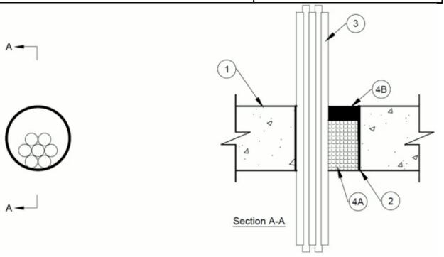
1. Floor or Wall Assembly — Min 4-1/2 in. (114 mm) thick reinforced lightweight or normal weight (100-150 pcf or  $1600 - 2400 \text{ kg/m}^3$ ) concrete. Wall may also be constructed of any UL Classified **Concrete Blocks\*.** Max. diameter of opening is nom 4 in. (102 mm).
