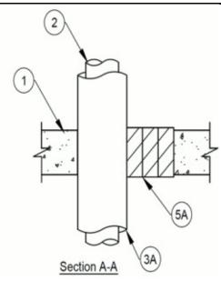
1. **Floor or Wall Assembly** — Min 4-1/2 in. (114 mm) thick reinforced lightweight or normal weight (100-150 pcf or 1600-2400 kg/m<sup>3</sup>) concrete. Wall may also be constructed of any UL Classified **Concrete Blocks\*.** Max area of opening is 384 in.<sup>2</sup> (2477 cm<sup>2</sup>) with a max dimension of 32 in. (813 mm).
