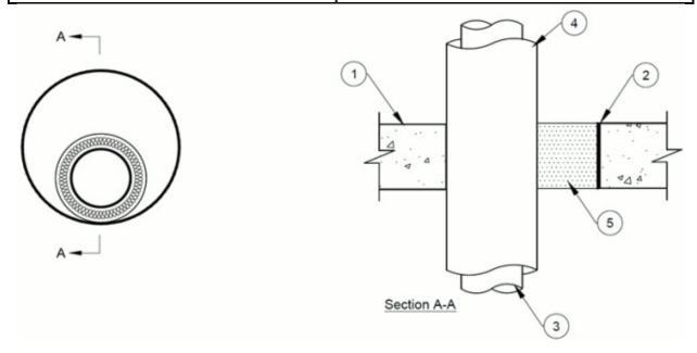
1. **Floor or Wall Assembly** — Min 4-1/2 in. (114 mm) thick reinforced lightweight or normal weight (100 - 150 pcf or 1600-2400 kg/m<sup>3</sup>) concrete. Wall may also be constructed of any UL Classified **Concrete Blocks\*.** Max diam of opening is 12 in. (305 mm).
