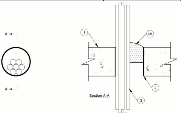
1. Floor or Wall Assembly — Min 4-1/2 in. (114 mm) thick reinforced lightweight or normal weight (100-150 pcf or  $1600 - 2400 \text{ kg/m}^3$ ) concrete. Wall may also be constructed of any UL Classified **Concrete Blocks\*.** Max diameter of opening is nom 5 in. (127 mm).
